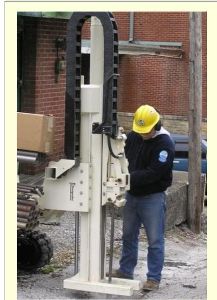
A geoprobe is used to collect a soil sample at an old hospital property. Phase II sampling can determine whether a release has occurred, delineate the extent of the contamination, develop a cleanup cost estimate and determine a baseline environmental condition for liability purposes.
